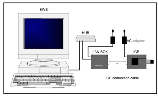
LAN-BOX : Unit used to connect the ICE to a LAN. It is provided with a 10BASE-T
