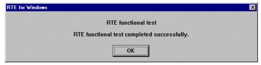
If an error occurs during the test, the user system has a failure or the JTAG/N-Wire cable is not properly connected. Check its connection.
