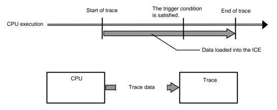
Figure 1 Flow of loading trace data
