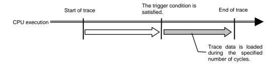
Figure 3 Flow of delay count
