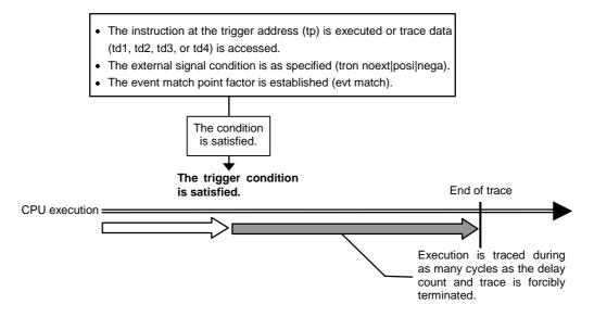
Figure 7 Trigger condition
